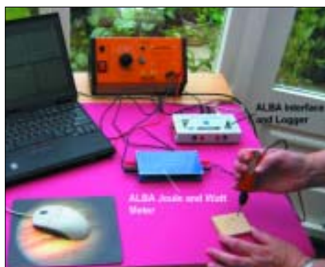
Figure 1. Investigating a drill on/off load with the ALBA Joule and Watt Meter.
