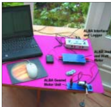
Figure 3. Investigating the efficiency of a geared motor with the ALBA Joule and Watt Meter.
