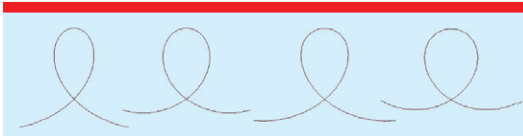
Figure 2. Different loop shapes for the condition of constant centripetal acceleration. The first two loop shapes give a centripetal acceleration of 2g and 3g , respectively, throughout the loop (for a particular velocity), whereas the last two loops maintain these conditions only for the bottom part of the loop, matched to a 120^\circ circular arc at the top. The loop with 3g centripetal acceleration throughout the loop is very similar to the Invertigo loop in figure 1.
