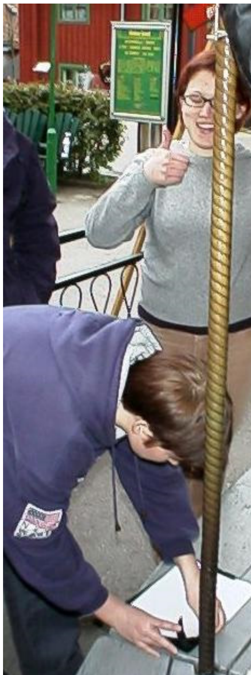
Figure 3. An experiment to measure the deviation of a falling marble when the carousel is in motion.
