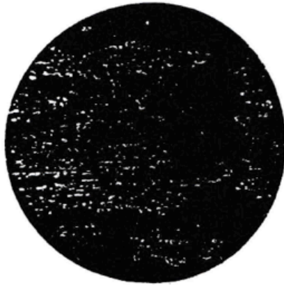
The earliest photomicrograph of a piece of wrought iron. Made by Henry Clifton Sorby in Sheffield in August 1864. Sorby's work showed conclusively that deformation did not destroy crystallinity.
