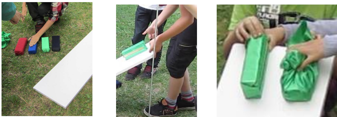
Figure 2: Blocks covered with different materials (a) and measurement of the slope where a block starts sliding (b). The photo in (c) shows a comparison between two blocks sliding with different sides toward the plane.
